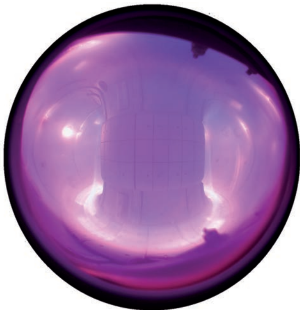
Obr. 8. Plazma v tokamaku COMPASS [2]
